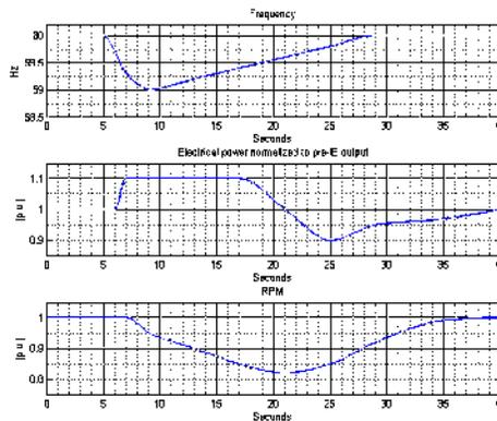
Figure 1 - Idealized ENERCON Inertia Emulation response to an under-frequency event at below-nominal, constant wind speed.
