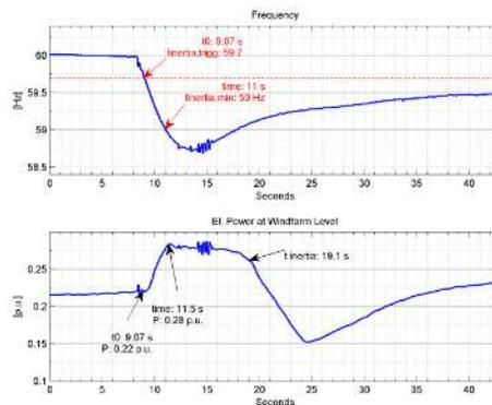
Figure 4 – Lower Power Band WPP measurement.
