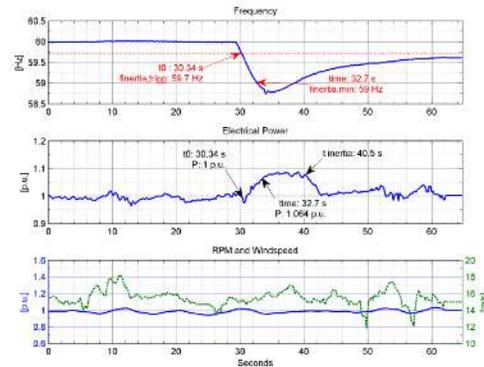
Figure 3 - Nominal power band WT measurement.
